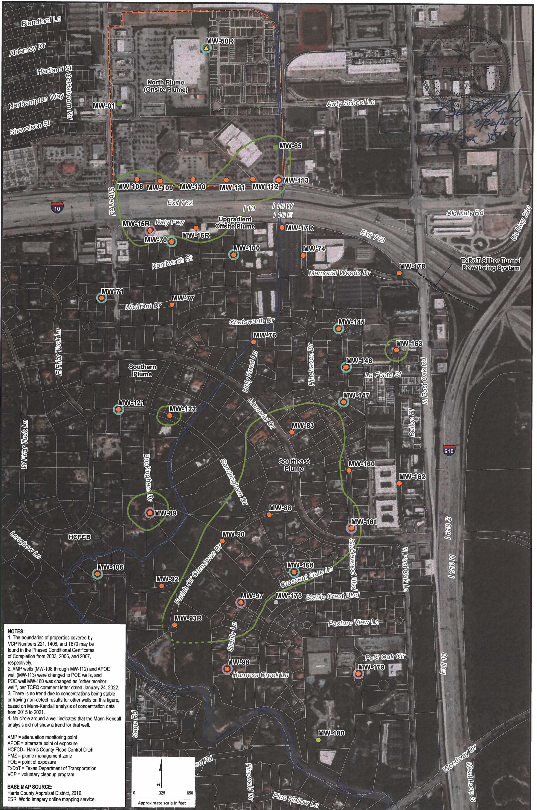
Legend ■ APOE Well ▭ Former Facility Boundary — TxDOT Dewatering System — 1,1-Dichloroethene cPCL Exceedance Boundary ▲ AMP Well ▭ PMZ Boundary ○ Increasing Mann-Kendall Trend - - - Dashed Where Inferred ● POE Well ▭ HCFCD ○ Decreasing Mann-Kendall Trend □ Parcel ● Plugged and Abandoned Well (2021) ▭ Gaining Portion of Stream ● Other Monitoring Well Figure 4-1c. Mann-Kendall Trend Map - 1,1-Dichloroethene 2021 Response Action Effectiveness Report Former Cameron Iron Works Facility, Houston, TX
