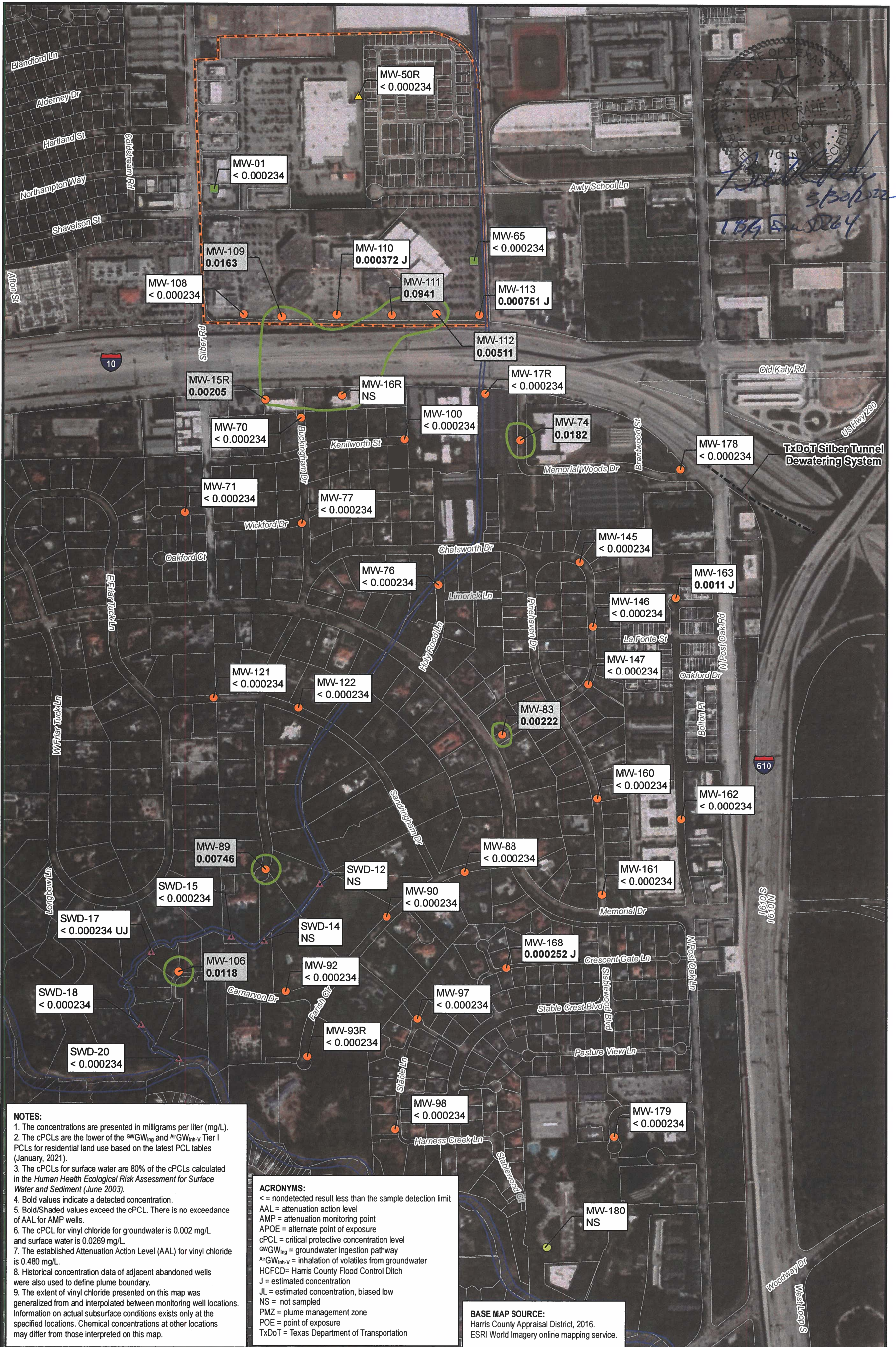
Figure 2-7. Vinyl Chloride Concentration Map 2021 Response Action Effectiveness Report Former Cameron Iron Works Facility, Houston, TX
